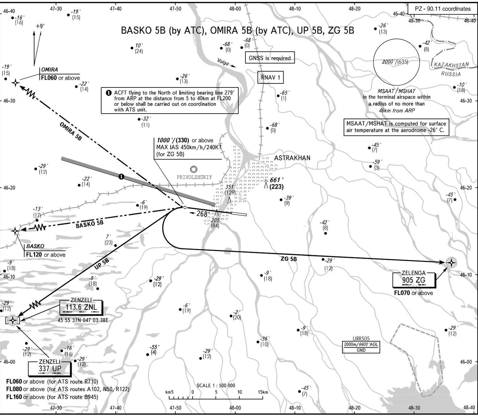
① ACFT flying to the North of limiting bearing line 279° from ARP at the distance from 5 to 40km at FL200 or below shall be carried out on coordination with ATS unit.
